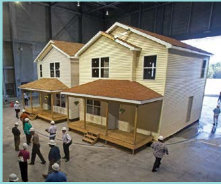
IBHS is the only lab in the world that can test full-scale one- and two-story residential and commercial buildings in a controlled, repeatable fashion for highly realistic windstorms, wind-driven rain, hailstorms and wildfire ember storms. Photos courtesy of Insurance Institute for Business & Home Safety
