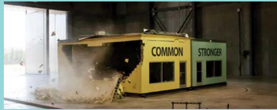
IBHS is the only lab in the world that can test full-scale one- and two-story residential and commercial buildings in a controlled, repeatable fashion for highly realistic windstorms, wind-driven rain, hailstorms and wildfire ember storms. Photos courtesy of Insurance Institute for Business & Home Safety
