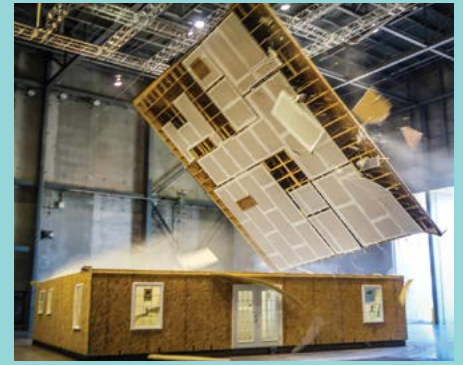
IBHS is the only lab in the world that can test full-scale one- and two-story residential and commercial buildings in a controlled, repeatable fashion for highly realistic windstorms, wind-driven rain, hailstorms and wildfire ember storms. Photos courtesy of Insurance Institute for Business & Home Safety
